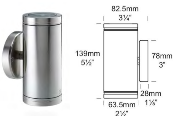
Product Name: Pillar Lite Designer: Hunza Manufacturer: Hunza IP: 66 Light Source: Halogen 2 x 20W MR16 or LED 2 x 6W Material: Aluminium, Copper and Stainless Steel Finishes: Black/Bronze/Copper/Corten/Grey/ Metallic Silver/Silver/Stainless Steel/White
