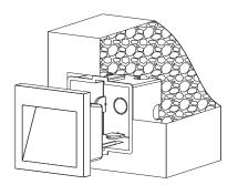
**2.** Connect wires in parallel and make sure all joins are made to keep the IP rating of the luminaire.
