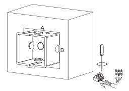
Cut a hole with the dimensions Ø 95mm (or 80 x 80mm for square) and fix canister into wall.
