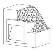
**3.** Insert luminaire into wall box.
