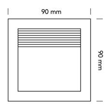
Depth: 25 mm Cut out: 77 x 77 mm
