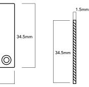
**Joining Clip** Code: 10-S30J (for both finishes)
