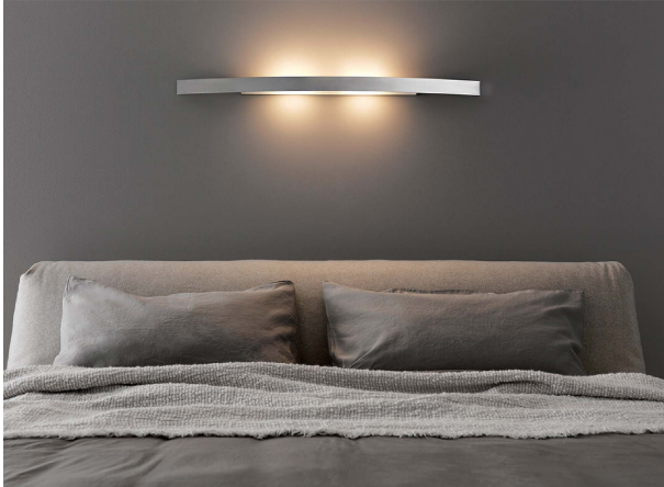
Product Name: Riga Designer: Paolo Zani Manufacturer: Fontana Arte IP: 20 Light Source: LED 2 x 9.5W, 2 x 80W R7, 3 x 120W R7 Material: Stainless Steel, Nickel & Aluminium Finishes: White, Stainless Steel or Satin Nickel
