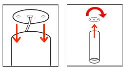
2 a) Pull cable through the ceiling mount and connect to fitting cables.b) Half turn twist the fitting to the base plate in the ceiling.
