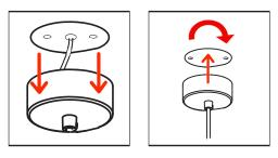
2 a) Pull cable through the ceiling mount and connect to fitting cables.b) Half turn twist the canopy into the base plate in the ceiling
