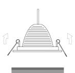
**STEP 3**Pull back springs and load unit into ceiling.
