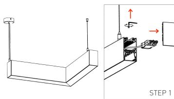
Remove end cap (both ends) and unscrew base to pull out the adapter.
