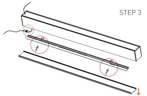
3. Remove LED heat sink by half turning in the 2 pictured locations and unhook heat sink cable.
