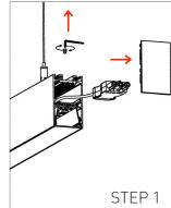
Remove end cap and unscrew base to pull out the adapter.
