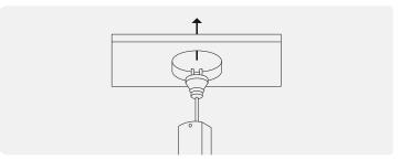
Connect the driver to the mains power socket - located in the ceiling cavity. Ensure the control gear is placed above any insulation.
