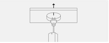
Connect the driver to the mains power socket - located in the ceiling cavity. Ensure the control gear is placed above any insulation.
