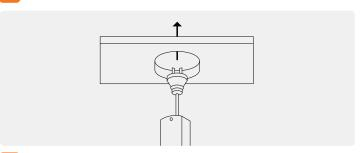
Connect the driver to the mains power socket - located in the ceiling cavity. Ensure the control gear is placed above any insulation.
