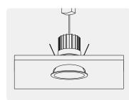
Pull back springs and load unit into ceiling.
