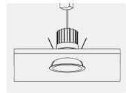
Pull back springs and load unit into ceiling.
