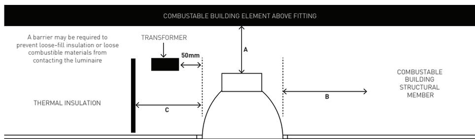
**A** Height clearance to building element (HCB) = **0mm**
