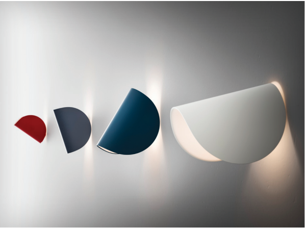
Product Name: IO Designer: Claesson Koivisto Rune Manufacturer: Fontana Arte IP: 20 Light Source: 2 LED – 4,5W – 700 K, CRI >80 Material: Aluminium Finishes: Blue, Graphite grey, Red or White
